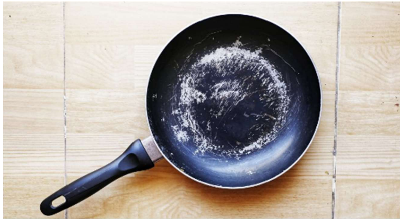
Figure 2: Scratches due to use of abrasive materials
