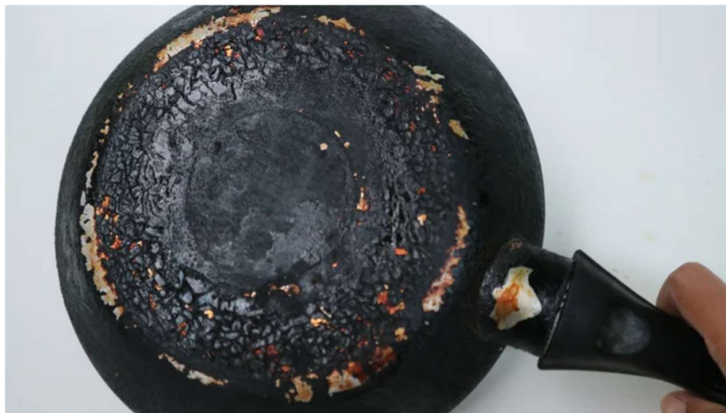
Figure 3: A pan damaged by excessive heating
