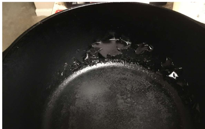
Figure 1: Peeling of the non-stick coating layer of the pan
