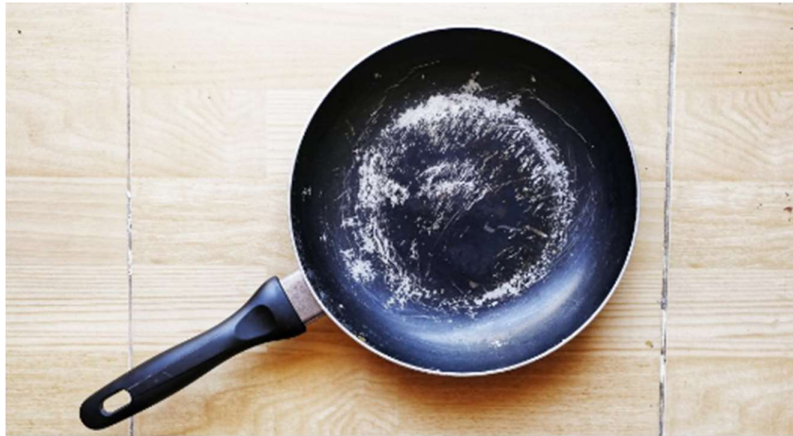
Figure 2: Scratches due to use of abrasive materials
