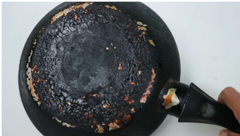
Figure 3: A pan damaged by excessive heating
